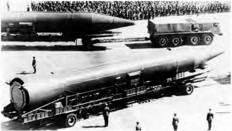
#21. R-14 (NATO SS-5) Intermediate Range Ballistic Missile (IRBM). Much larger and longer range than the R-12 MRBM. (Image source: Wikipedia.)
